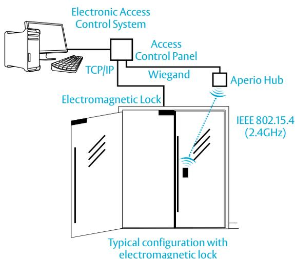
Local wireless communication eliminates the cost and inconvenience of wiring in and around the door, without the hassle of complex site surveys.
