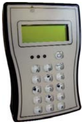
DTD (Data Transfer Device)
